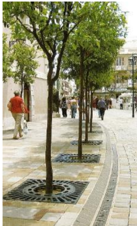
Integrated tree grilles and drainage
